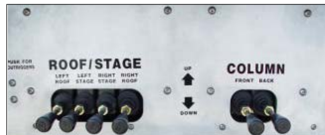
Figure 5.5 — Roof Raise and Tilt Controls
