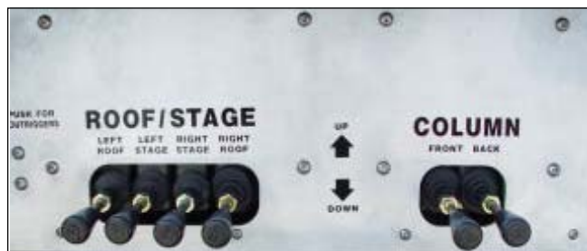
Figure 5.10 — Roof Raise and Tilt Controls
